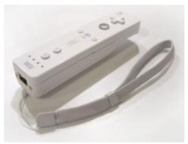
The Wiimote communicates with the Wii via a Bluetooth wireless link. The Bluetooth controller is a Broadcom 2042 chip, which is designed to be used with devices which follow the Bluetooth Human Interface Device (HID) standard, such as keyboards and mice. The Bluetooth HID is directly based upon the USB HID standard, and much of the same documentation applies.
